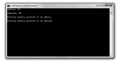
**Figure 9.3** The two int values are stored on the heap.
