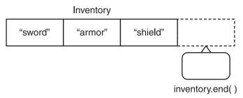
**Figure 4.4** A call to inventory.end() returns an iterator one past the last element of the vector.
