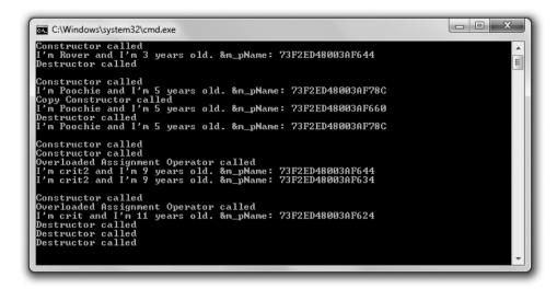
**Figure 9.6**Objects, each with a data member that points to a value on the heap, are instantiated, destroyed, and copied.
