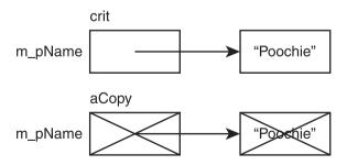
**Figure 9.10**With a proper copy constructor, the original and the copy each point to their own chunk of memory on the heap. Then, when the copy is destroyed, the original is unaffected.
