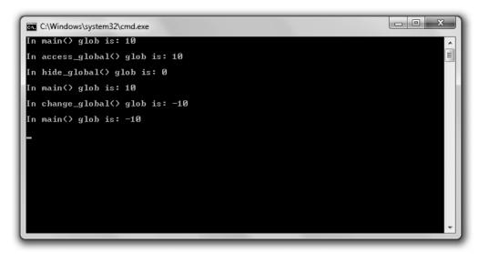
**Figure 5.4**You can access and change global variables from anywhere in a program—but they can also be hidden in a scope as well.
