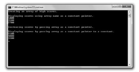
**Figure 7.8**Using an array name as a pointer, the high scores are displayed, altered, and passed to functions.
