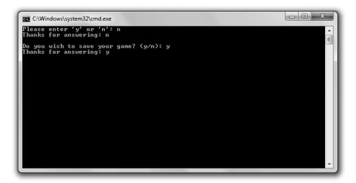
**Figure 5.2** Each question is asked by a separate function, and information is passed between these functions and main().
