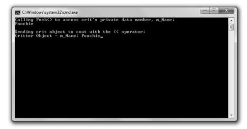
**Figure 9.2**The name of the critter is displayed through a friend function, and the critter object is displayed by sending it to the standard output.
