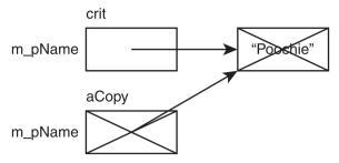
**Figure 9.9**If the shallow copy of the Critter object were destroyed, the memory on the heap that it shared with the original object would be freed. As a result, the original object would have a dangling pointer.
